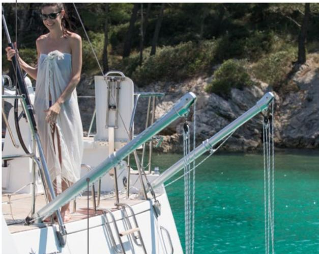
Retractable davits allowing launching of a big dinghy without taking inside space. They disappear when are not in use.
