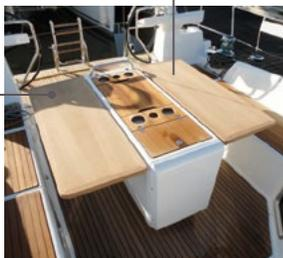
A “safety first” conception ensuring easy deployment of the liferaft at the end of the table without necessity of opening the transom
