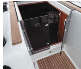
Companionway hatch with hinged double doors
