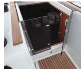
Companionway hatch with hinged double doors
