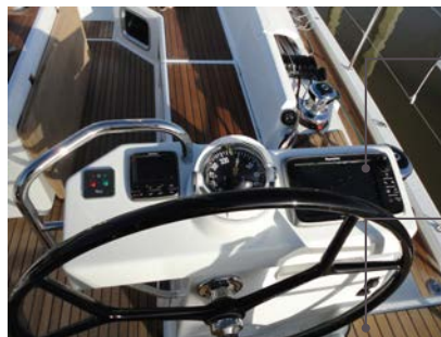
GPS integrated into a pod
