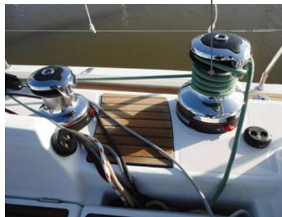
All the winches are located ahead the helm stations in order to ensure easy sail handling and frees up the rest of the cockpit
