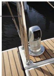
Retractable davits allowing launching of a big dinghy without taking inside space. They disappear when are not in use (maximum weight 120kg)
