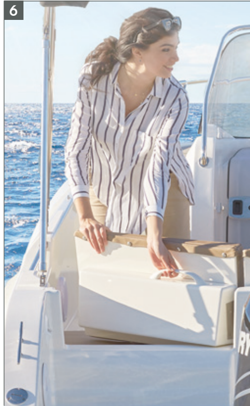
Port and starboard pivoting backrest allowing an easy access to the swim platforms
