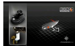
> Sideways movement: saildrive turns 90° and activates bowthruster
