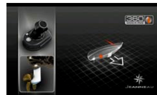
> Sideways movement: saildrive turns 90° and activates bowthruster
