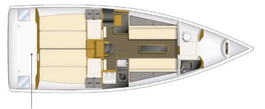
Storage lockers accessible from the deck hatches in the cockpit
