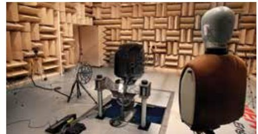
Mercury's Sound Lab is where our engineers analyze and optimize sound quality in order to achieve world-class noise, vibration and harshness (NVH) levels.
