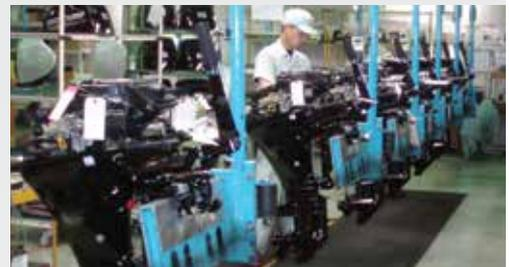
Following testing, technicians install the propeller and top cowl, then make final quality checks before the engine is boxed, assuring the ultimate in reliability.
