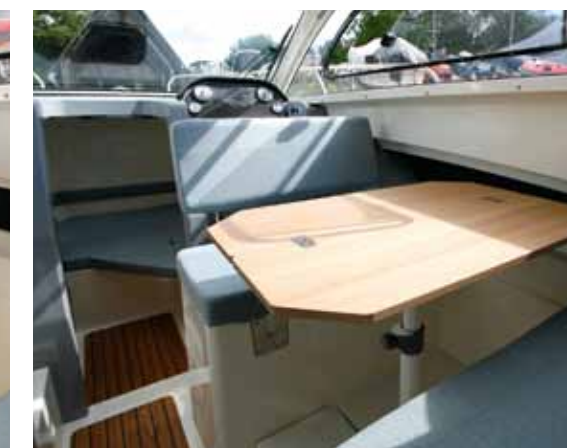
The helm seat backrest reverses to create a useful dinette with a folding table
