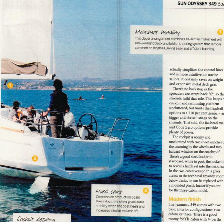
She's a small boat for twin wheels, but the helm position is well thought out with a footblock and seat moulded into the coaming Main and jib sheets run through a lead eye on the coachroof, on a Dyneema bridle
