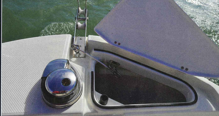
The position of the chain locker and windlass allows one to stand to one side to coil the warp down in the locker
