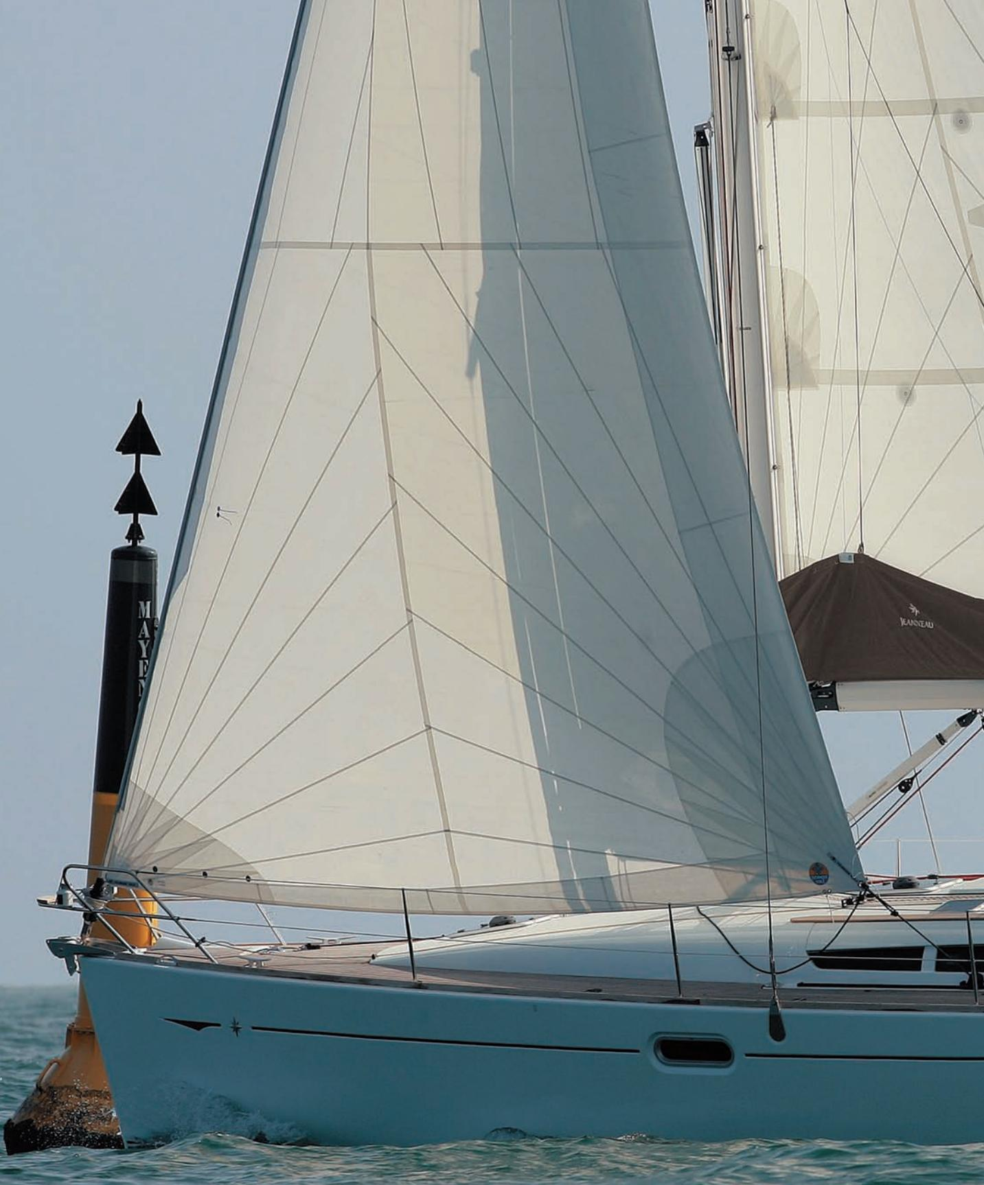
The Performance version of the Sun Odyssey 42i is designed for even more power and speed, fitted with Prestige series sails, tri-radial cut in Mylar/Taffeta, a taller mast, twin groove furler, a feathering propeller and more, allowing you to go faster while enjoying the same comfort offered on the standard version.
