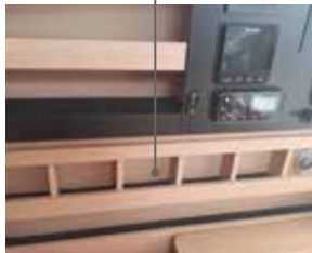
Sound deadening lining in cabinets
