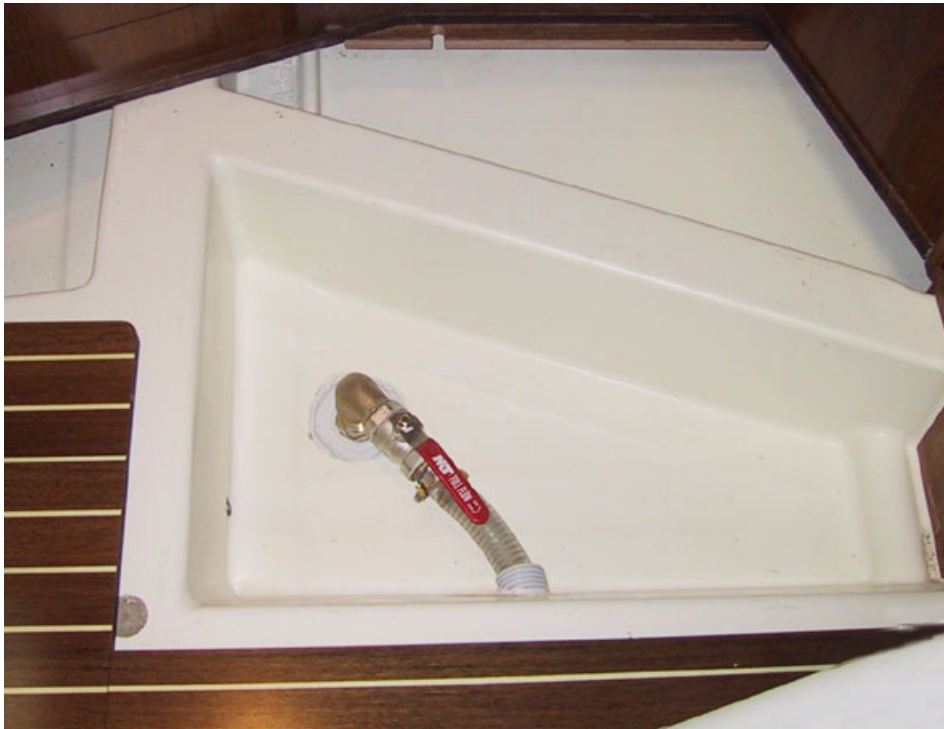
Thru-hull fitting with engine water inlet valve
