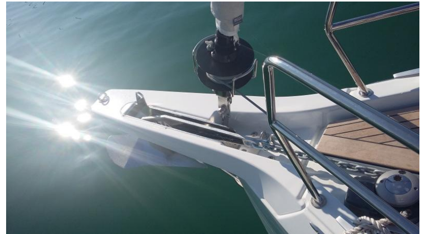
GRP bowsprit integrated stainless steel anchor roller
