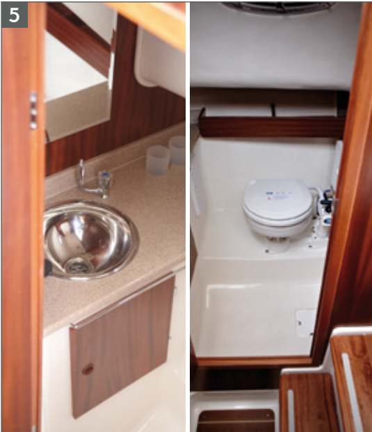
5 Enclosed sea toilet and lavatory sink
