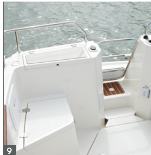
9 Transom door to ease access in and out of the boat
