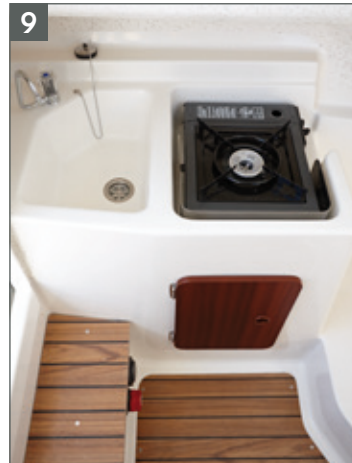
Galley with cold water sink and portable butane stove
