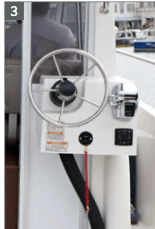
Optional second helm station to allow driving from the cockpit
