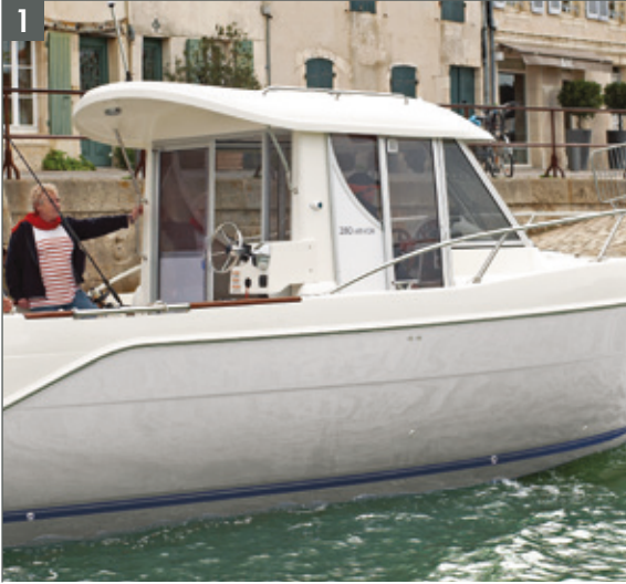
1 Asymmetric wheelhouse with a wide and safe passage to the bow on starboard
