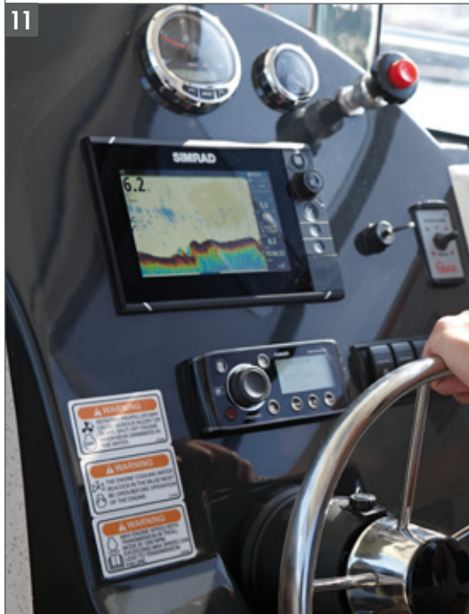
Integrated helm with hydraulic steering, SmartCraft instrumentation and optional 7" GPS and Bluetooth stereo
