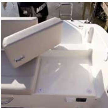
Super-clever hinged backrest aids access to the port-hand platform
