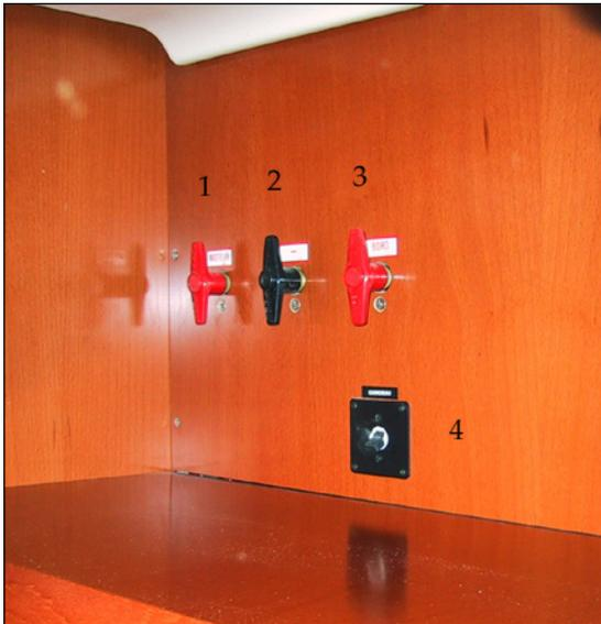
1. Battery switch + Engine
