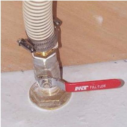
Thru-hull fitting **closed**
