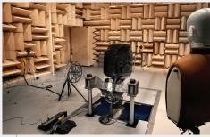
Mercury's hemi-anechoic chamber enables our engineers to analyze and optimize sound quality in order to achieve world-class noise, vibration and harshness (NVH) levels in our outboard engines.
