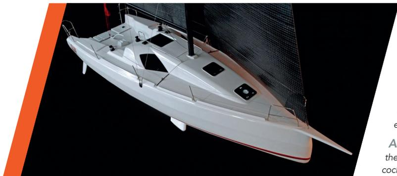
**A modern, innovative hull:** The double concave profile forward and aft offer a more balanced distribution of pressure. This reduces the overall drag, while minimising the wetted surface area. The inverted bow, in combination with tumblehome yields weight savings and notably lowers her centre of gravity, all while conserving her considerable strength.
