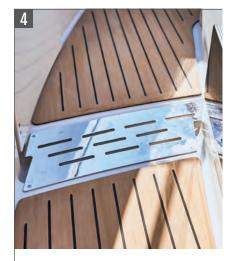
Drain system to avoid water accumulation
