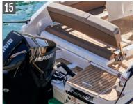
Large swim platforms and motor well step for easy access to both sides of transom
