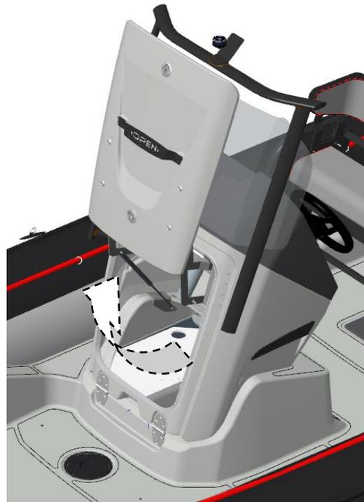
Unlock the two latches with the key **1** and use them to lift the console door.
