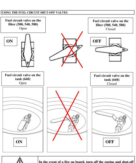
In the event of a fire on board, turn off the engine and shut-off the fuel circuit valves.
