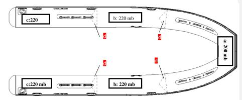
Inflation is completed: Screw on the inflation valve plugs.
