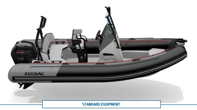
HULL & DECK: 1 Bow Bitt / 2 Aft Cleats , 1 Bow D Ring / 2 Towing Rings , 2 Bailers, Fairleads, GRP Deep V-Hull, Lockable Mooring Storage, Ski & Wakeboard Locker, Tilting Console.
